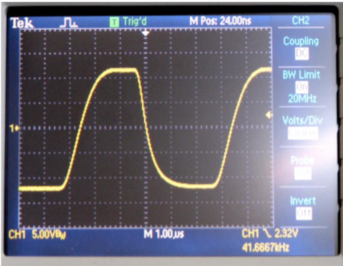
Note that the scope says it's 41.6667 kHz because the clocking program was 1000 cycles in 6 ms followed by 18 ms idle time. At 167 kHz, components get very hot when clocking continuously.
